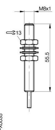
Inductive Sensors BES 516-324-SA 8-02 M8x1 x 55.5 normally-open Sn=1mm shielded temperature rated
